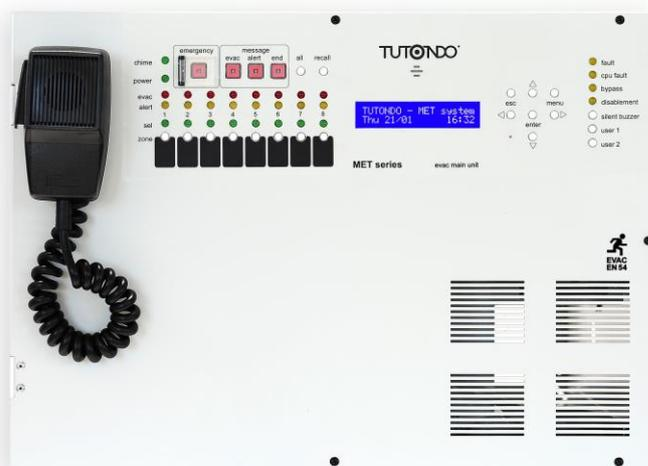
The system is designed for **connecting up to 8 power amplifier** (zones). Each amplifier drives a single lines speakers (or double lines with optional interface).
